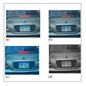
FIGURE 1. (a) original image (b) after applying minimum filter (Note that the diagonal strips passing through characters and edges of the plate disappeared, and the characters became bold and their area are increased, This is important in order to have many strong edges around the characters) (c) after increasing saturation (d) after converting to grayscale
