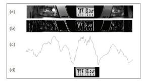
FIGURE 3. (a) band image; (b) after Sobel vertical edge detection; (c) horizontal projection for image (b) (Note that there are three peaks that corresponds to the left and right lamp and the plate); (d) the plate that corresponds to the middle peak
