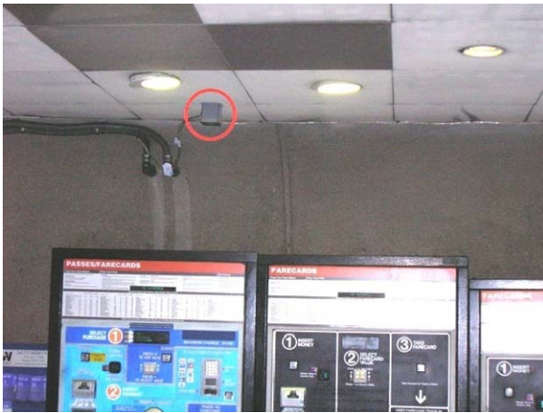
Figure 5. One of three cameras (circled) deployed in a test installation of the GammaPix technology at the Medical Center Station of the Washington, D.C., Metro system.
