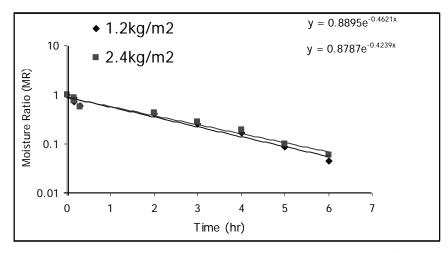
Fig. 2. Effect of loading density (Cubes) on drying rate at 55°C
