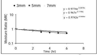
Fig. 4. Effect of thickness on drying rate at 50°C
