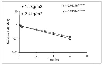
Fig. 3. Effect of loading density (Slices) on drying rate at 55°C
