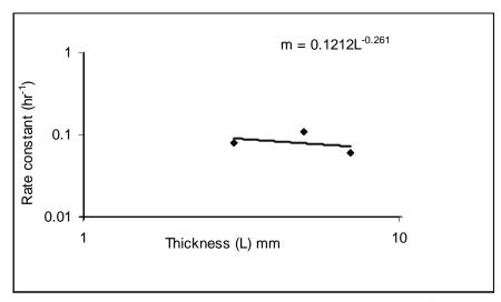
Fig. 5. Influence of thickness on drying rate constant at 50°C
