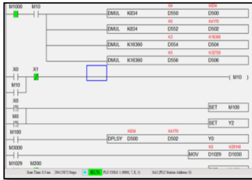
Fig 9: Ladder Diagram Indicating Pulse and Frequency
