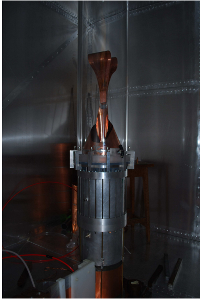
Figure 1 Non-invasive PEF system installed in Loughborough laboratory. Note the vertical plastic tube surrounding the antenna and filled with water
