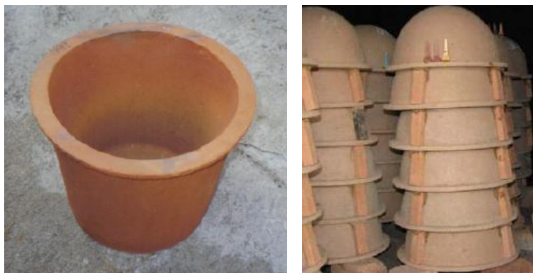
FIGURE 3 FLAT-BOTTOM CERAMIC WATER FILTER VS ROUND-BOTTOM FILTERS 36
