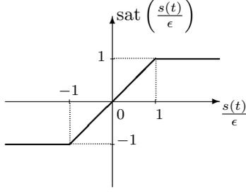
Fig. 2. Saturated function:  $\text{sat}\left(\frac{s(t)}{\epsilon}\right)$
