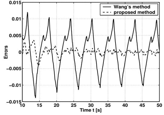
Fig. 3. Error signals of Case 1.
