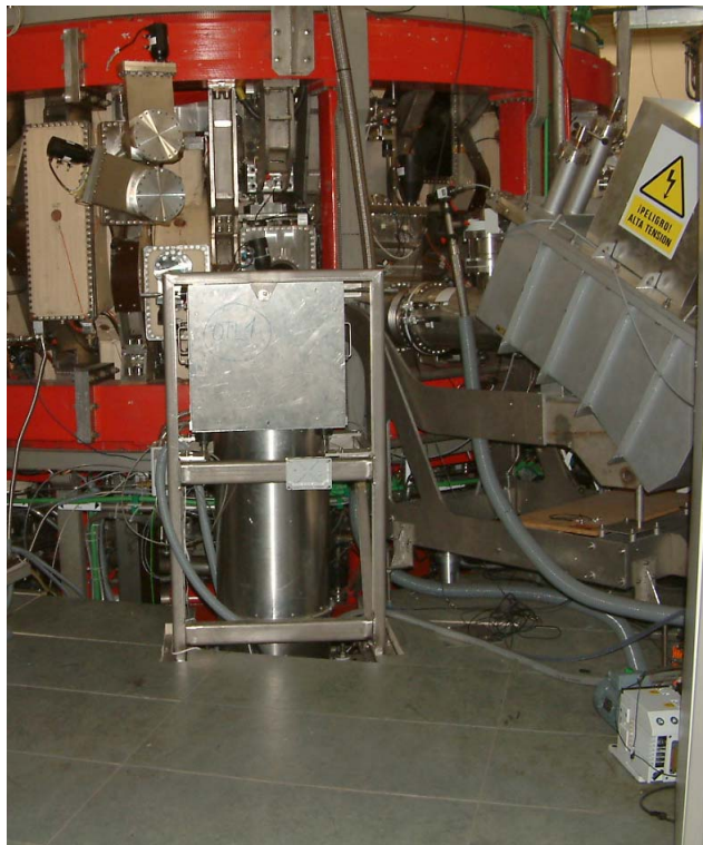
Figure 3: Photo of sector B3 showing the side access port and QTL support structure plus shielding.
