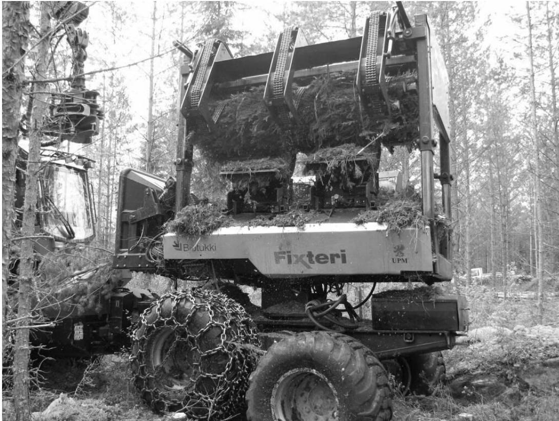
Figure 2. Fixteri whole-tree bundler at work. Photo: Kalle Kärhä/Metsäteho Oy.
