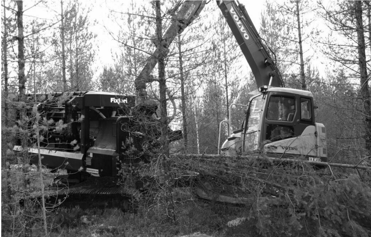
Figure4 . Fixteri bundler can also be mounted on an excavator. Photo: VTT.
