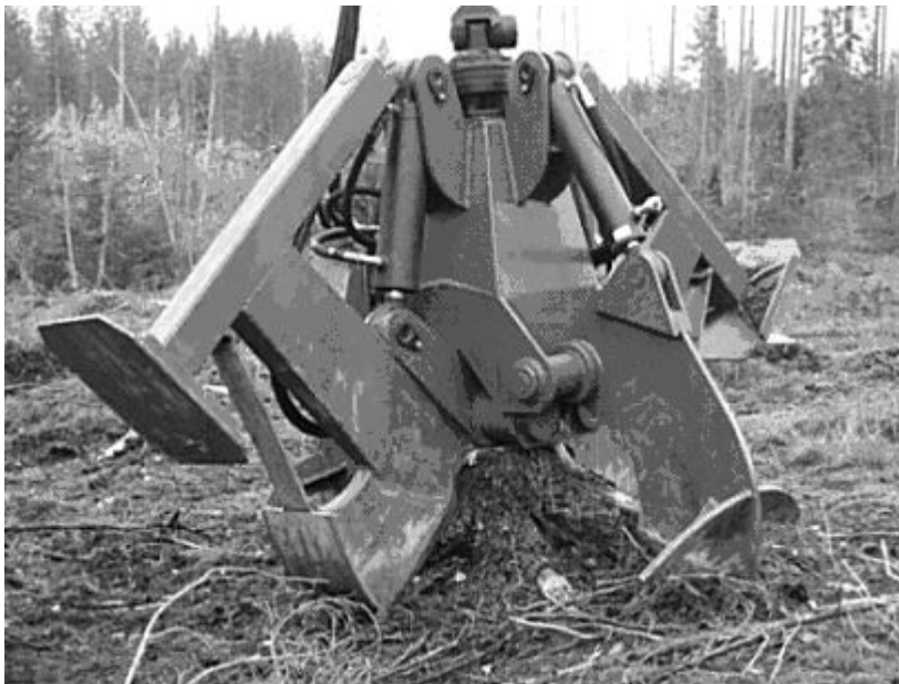
Figure 6. A new stump lifting and splitting device by Karelian Puu ja Metalli Oy. Photo: Dominik Röser/Metla.
