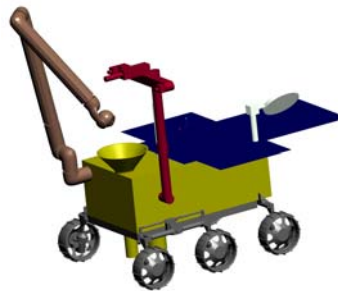
Figure 21: Six-wheeled rover with manipulation system for deploying instruments on lunar surface and for collecting regolith to fill ISRU demonstrator ovens.
