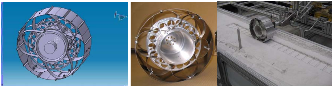
Figure 19: ExoMars Phase B1 conceptual flight design of metallic flexible wheel (left), view of corresponding Breadboard wheel (center), and wheel undergoing single wheel test (right).
