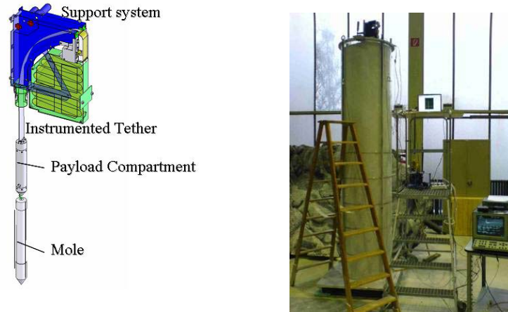
Figure 6: Schematics of the HP 3 instrument showing the functional subsystems (left). HP 3 Breadboard during 2.3 m soil intrusion test. The Support System is positioned at the top of soil cylinder (right).
