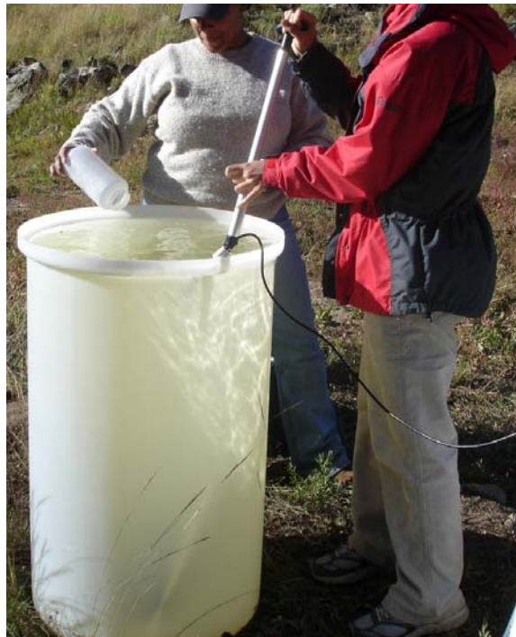
Figure 4. Lithium chloride was added to the injection solution and stirred with a paddle for 90 min until the salt was completely dissolved.
