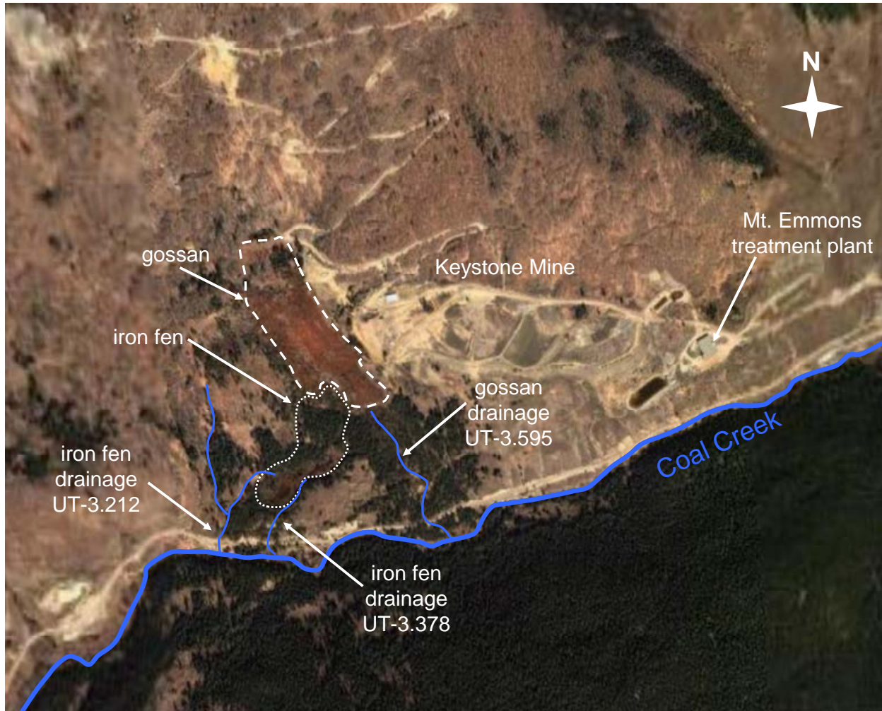
Figure 3. Aerial view of Coal Creek near the Keystone Mine at the base of Mt. Emmons, including the gossan located just west of the Keystone Mine, the iron fen, unnamed tributaries at stream distances of 3.212, 3.378, 3.595 km downstream of the injection site used for this study, and the Mt. Emmons treatment plant. Coal Creek flows to the northeast. The aerial photo was retrieved using Google Earth™ ( http://earth.google.com ).
