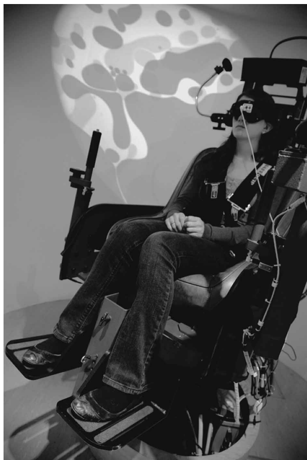
Figure 4. Motorized rotating chair (off-axis) with colourful moving pattern to keep child entertained between tests.
