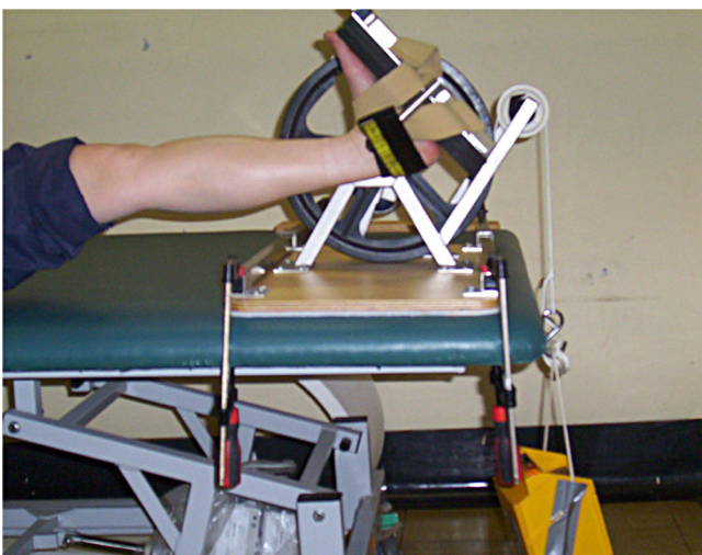
Figure 1. The device used to measure passive ankle dorsiflexion.
