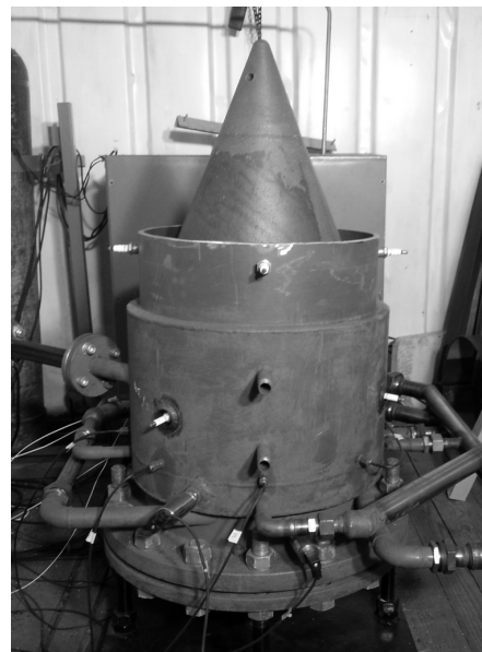
FIGURE 2. Continuous detonation combustor operating on hydrogen and air.
