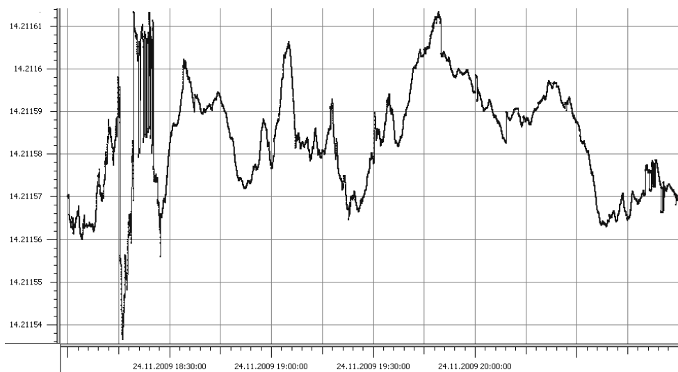
FIGURE 9. Positioning deviations in W-E direction from the Barentsburg station data in November 24, 2009.
