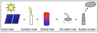
Figure 5 An energy balance for a solar water heater
