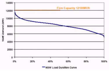
Figure 3 Low capacity factors do not reward large investments in electricity network augmentation. Data shown for NSW
