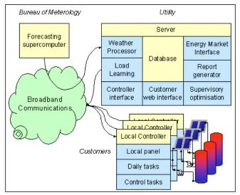
Figure 6 Distributed intelligence architecture for domestic hot water systems
