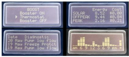
Figure 7 Four images of display options from the local controller
