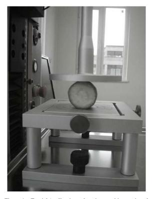
Figure 1 Zowick/roell universal testing machine equipped with a 500 N load cell
