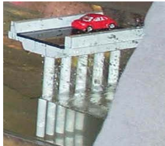
FIGURE 2 A BRIDGE PIER INSERT WITH REMOVABLE PIERS
