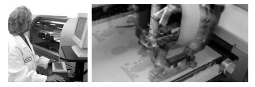
a) b) Figure 2. Prometal 3DP process: a) RP workstation, b) 3D printing [3]
