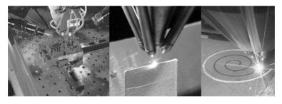
a) b) c) Figure 1. Directed Metal Deposition: a) RP workstation, b) i c) creating layers [2]
