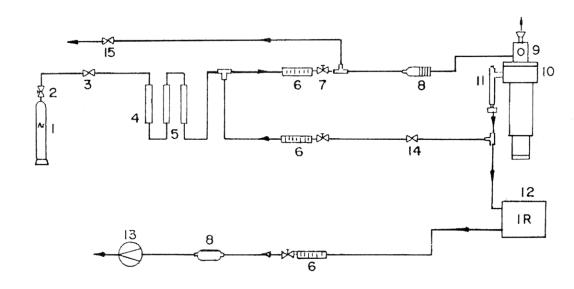
I carrier gas (argon) 2 reducing valve 3 solenoid valve 4 NaOH trap 5 Mg(ClO4)2 trap 6 flow meter 7 regulating valve
