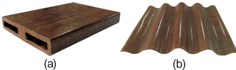
Figure 8. Profiling (a) and roof (b) made from bamboo composites reinforcement thermoplastic.
