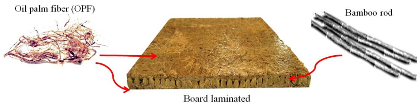
Figure 6. Samples of hybrid biocomposites board. Oil palm fiber laminated with bamboo rod.
