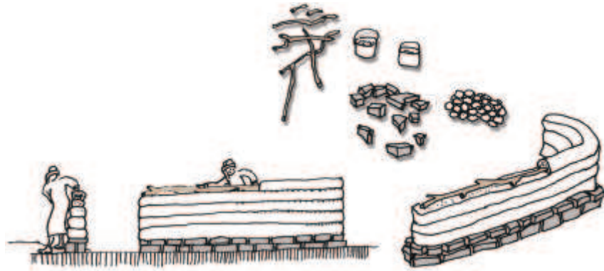
Figure 3. Sketches of elements to reinforce the wall capacity to bear the load and to achieve higher resistance. Enveloped wood in the wall construction is well preserved from insects and mould (drawing by author).
