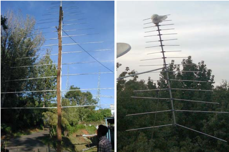
Fig. 3 Logarithmic periodic antennas of e-CALLISTO. Left: at Ootacamund (Ooty) in Tamil Nadu, India; Right: at UNAM, Mexico D.F.
