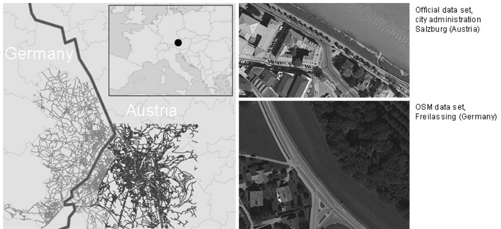
Fig. 4: Location of the study area (left) with different data sources. The data model of the official data (dark green/grey) and OSM (light green/grey) are fundamentally different (right): e.g. separated lanes are geometrically represented in the OSM data, whereas in the official data set they are attributes of the centre-line edge.
