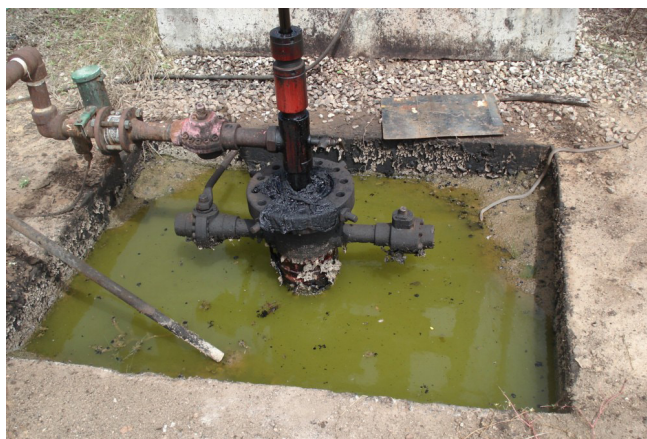
FIGURE 1: The accumulation of water mixed with crude oil at the ground of an oil extraction well.
