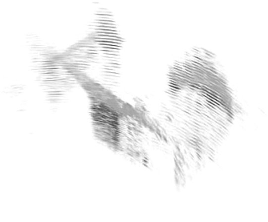
Figure 3. A 3D point cloud, representing the reflected acoustic intensity of each point in greyscale, of an underwater arch produced by the Tritech Eclipse Multi-beam Sonar.
