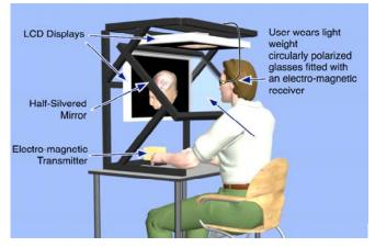
Figure 3: Schematic of the ImmersaDesk-4.
