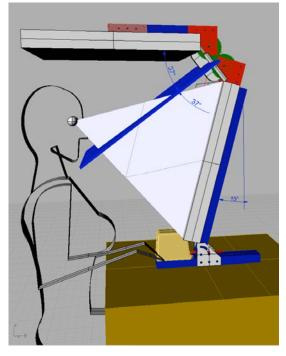
Figure 4: An Early Prototype Design of the ImmersaDesk-4. This version was actually built but was found to be structurally unstable.
