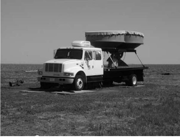
Figure 2. Photo of the University of Massachusetts S-Band FMCW radar system mounted on flatbed truck. Electronics are contained within the cab.
