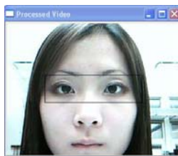
Figure 2. Driver positions her eyes in the calibration box, in preparation for ‘freezing’ the open and closed eye-state templates.
