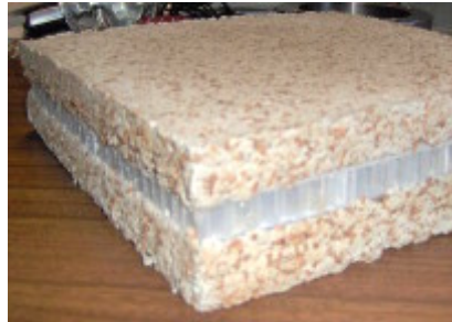
Figure 9. Sandwich panel made from a paper pulp/cork plate and PP honeycomb
