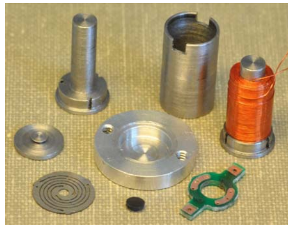
Figure 12: The Actuator of the LTCC integrated valve
